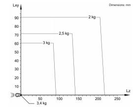
The LBR iisy 3 R760 is designed for a rated payload of 3 kg in order to optimize the dynamic performance of the robot. The maximum payload of 3.34 kg only applies if the position of the center of mass is 0 mm. The specific load case must be verified using KUKA.Load or KUKA Compose. For further consultation, please contact KUKA Support.
